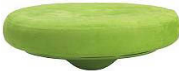
Figure 6: The Virrig input device shown from the side. It is very flexible in use as the user can sit, stand, kneel or lie on it and it is very robust.
