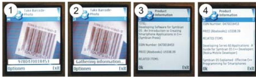
Figure 6: Example application : The above screenshots show a literature information system – sample application implemented using our recognition and resolution system.
