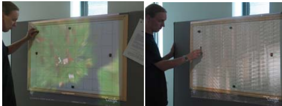
Fig. 6. The zoom dial quickly repositioned (left) and trying out a slider for panning (right)
