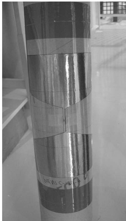
Fig. 5. C-tag antenna mounted on the reel core.
