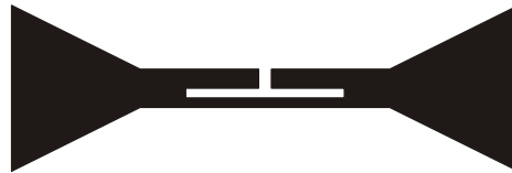
Fig. 1. Structure of a bow-tie antenna that is designed to operate through paper.
